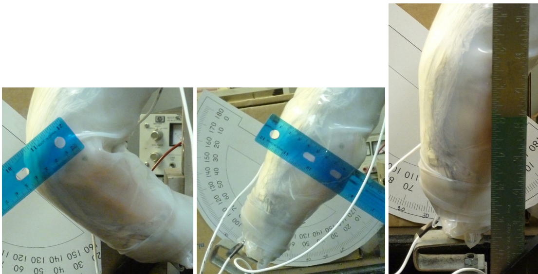
Figure 4.10: Measurements of test stand dimensions relative to axis of rotation (top: flexion and extension; bottom: length of pendulum).
