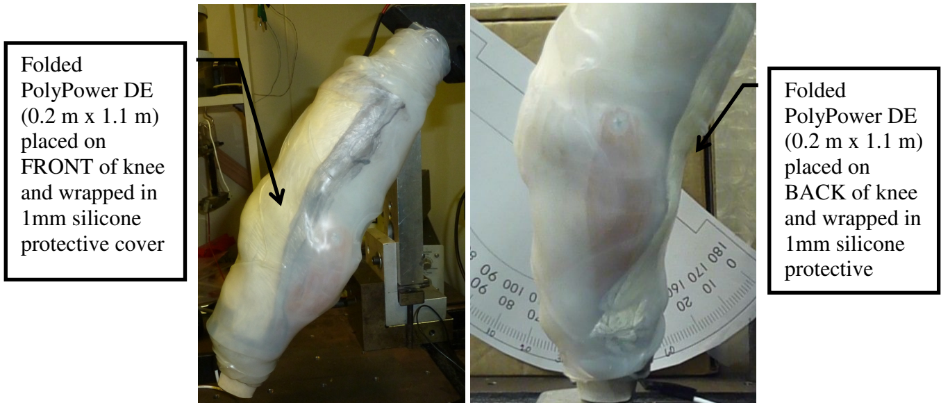
Figure 4.13: DE film placement on the knee joint test stand; left -- front of knee joint, right -- back of knee joint.
